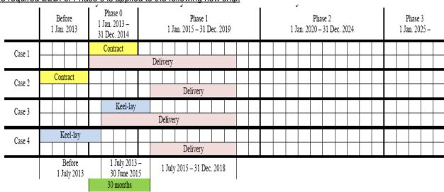
The required EEDI of Phase 1 is applied to the following new ship:
