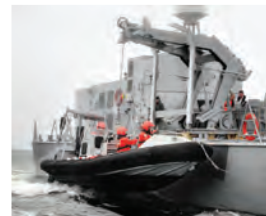
Rescue and Towing Ship / Istanbul Shipyard High Speed Rescue Boat Davit Gurdesan Gemi Makinalari San. Ve Tic. A.S. GD-HBMA 35/5.0 - PG A Davit
