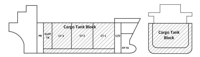
Cargo tank block is the part of the ship extending from the aft bulkhead of the aftmost cargo or slop tank to the forward bulkhead of the forward most cargo or slop tank, extending to the full depth and beam of the ship, but not including the area above the deck of the cargo or slop tank.
