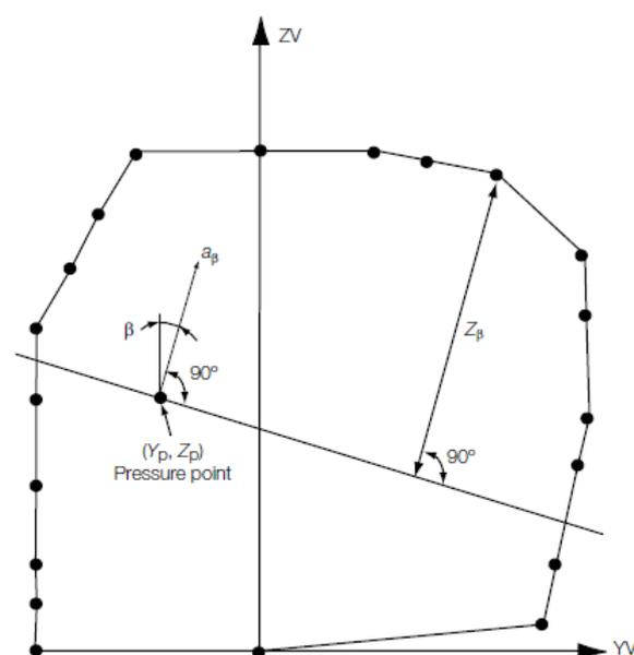
Fig.2 Determination of internal pressure heads
