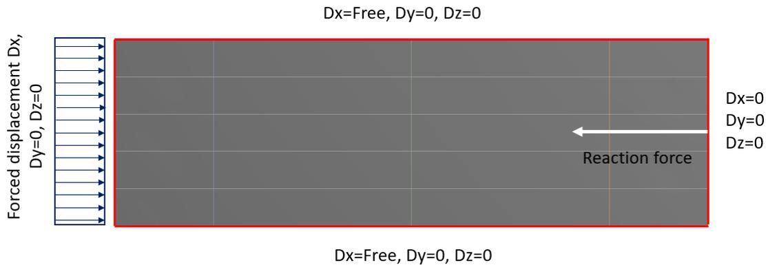
Figure 4.2: Method of load application
