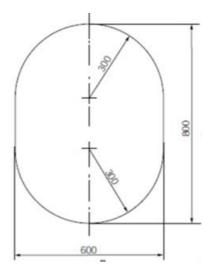
2. Subject to verification of easy evacuation of injured person on a stretcher the vertical opening 850 mm x 620 mm with wider upper half than 600 mm, while the lower half may be less than 600 mm with the overall height not less than 850 mm is considered an acceptable alternative to the traditional opening of 600 mm x 800 mm with corner radii of 300 mm.
