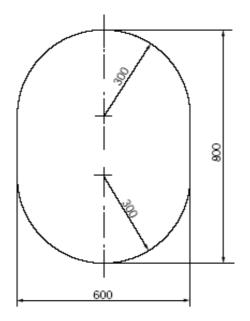
.3 Circular access openings in type-C cargo tanks should have diameters of not less than 600 mm.
