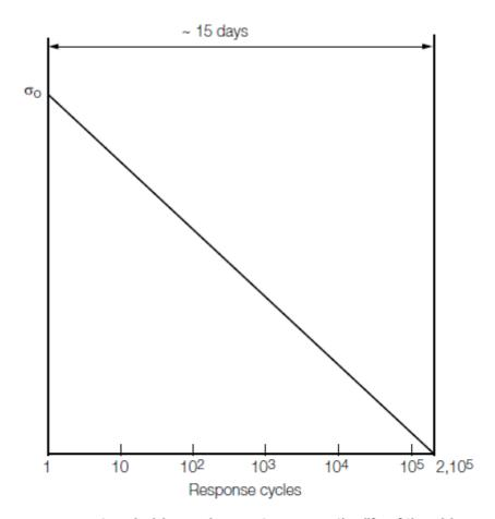
$\sigma_{\rm O}=$  most probable maximum stress over the life of the ship Response cycle scale is logarithmic; the value of 2,10 $^{5}$  is given as an example of estimate
