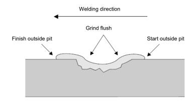
Figure 2.7 Welding of pits
