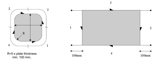
Figure 2.2 Welding sequence for inserts
