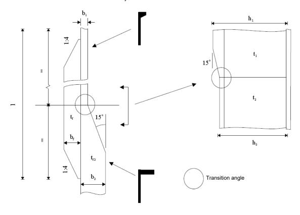
Figure 2.5 Transition between inverted angle and bulb profile
