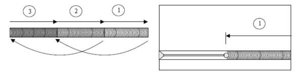
Fig.2.10 Welding sequence for cracks with length less than 300 mm.
