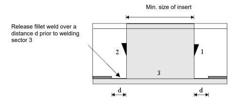
Figure 2.4 Welding sequence for inserts of stiffeners
